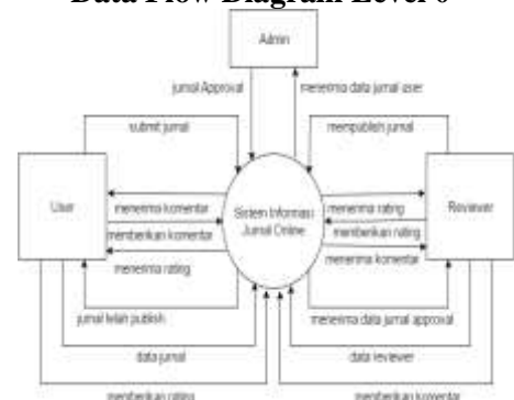
Gambar 2 Data Flow Diagram Level 0
